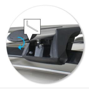
• Tighten adjusting screw to 5 Nm.
