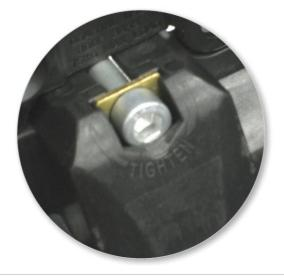
Bolt should sit in groove as shown.
