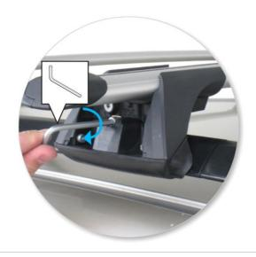
Use 5 mm Allen Key to tighten clamp and secure crossbar to rail.
