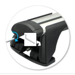
• Tighten adjusting screw to 5 Nm.
