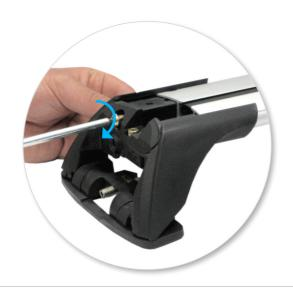
• Tighten adjusting screw to 5 Nm.
