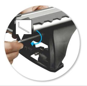
Once roof racks have been fitted to the vehicle, tighten adjusting screw to 5 Nm.
